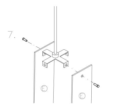
Attach the 2 narrow (2" wide) glass pannels () first **Pannel should hang freely, do not over-tighten**
